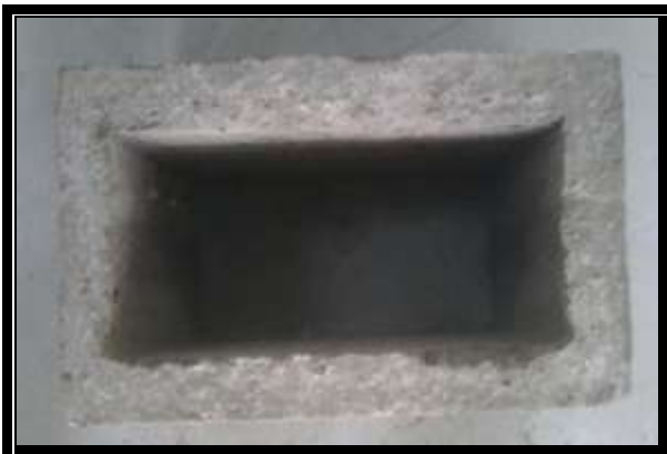
Figure 2: Ferrocete confinement specimen without concrete infill
