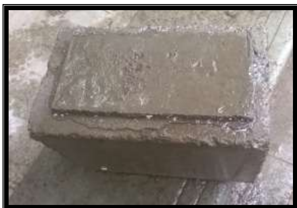
Figure 3: Ferrocete confinement specimen with concrete infill
