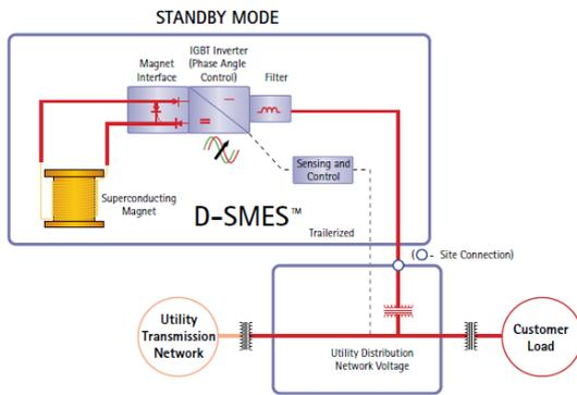
Figure 1: Shows a schematic of D-SMES unit.
