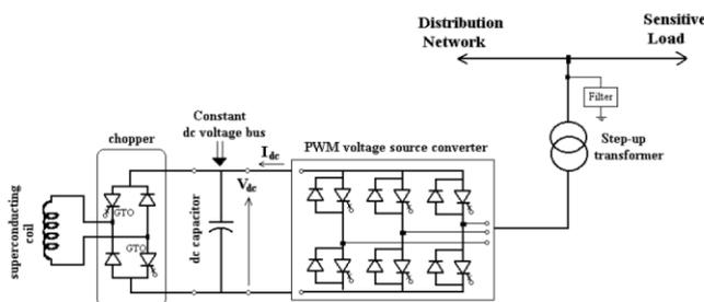
Figure 2: Simplified D-SMES one-line diagram
