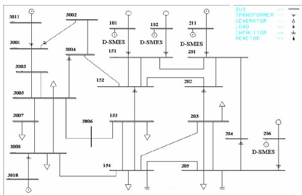
Figure 3: Diagram of the sample system
