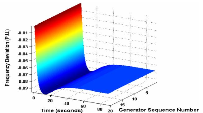
Figure 5. The frequency dynamics of all the buses in the system when Gen.101 is tripped.
