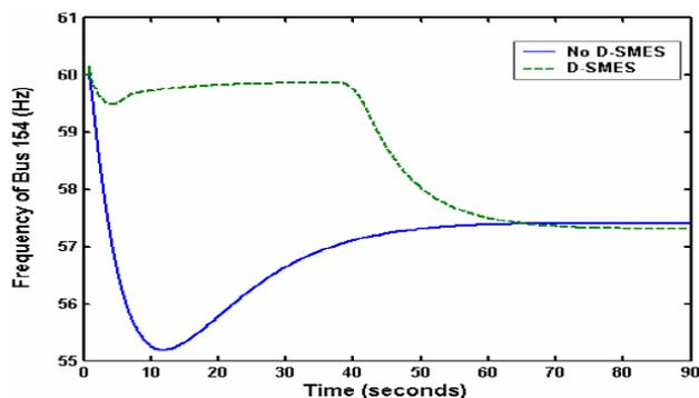
**Figure. 7.** Comparison of frequency of bus 154 when Gen.211 is tripped.
