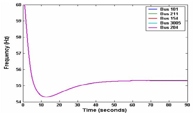
Figure 4. Frequency of different buses when generator at bus 101 is disconnected.
