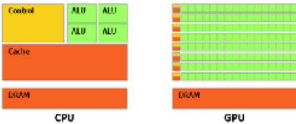
Figure 1: Design philosophies of CPU and GPU
