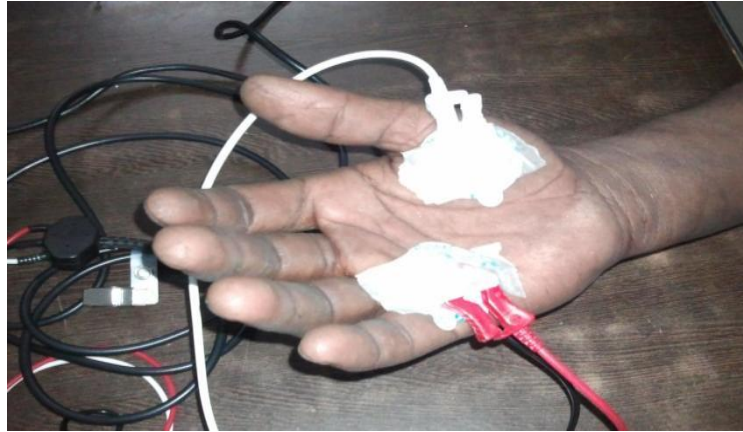
Figure 3.1: Electrodes placement during the EMG data collection
