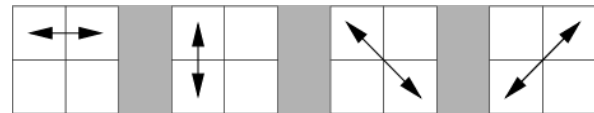
Fig 4: Four directions of adjacency as defined for calculation of the Haralick texture features.
