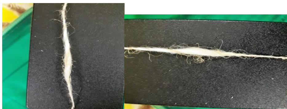
Figure 5.3: Thick Place and Irregular distribution of Polyester Fiber in Blend Yarn
