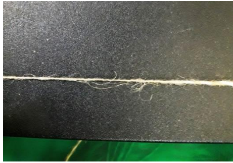
Figure 5.5: Thin Place in Blend Yarn
