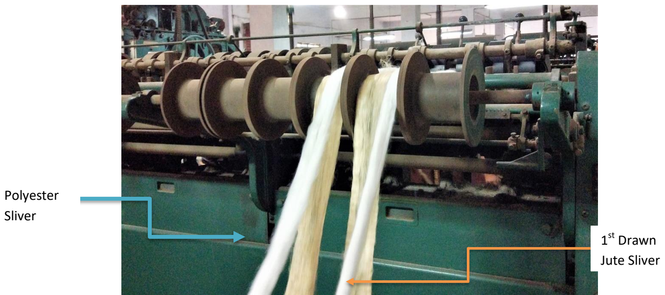
Figure 4.9: Blending of Jute with Polyester in 2 nd Draw Frame
