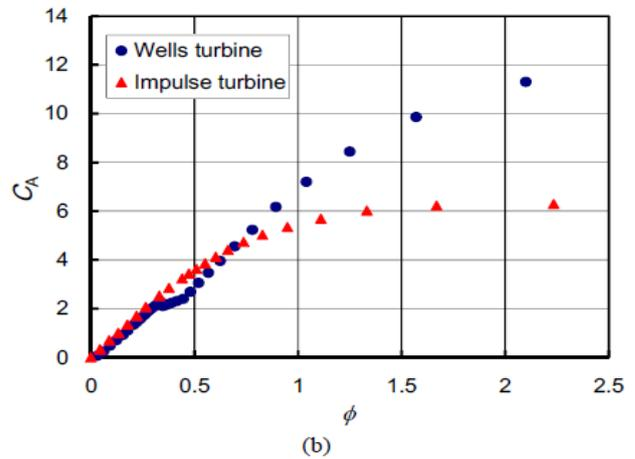
**Figure 7:** Turbine characteristic under unfluctuating stream condition: (b) Input Coefficient
