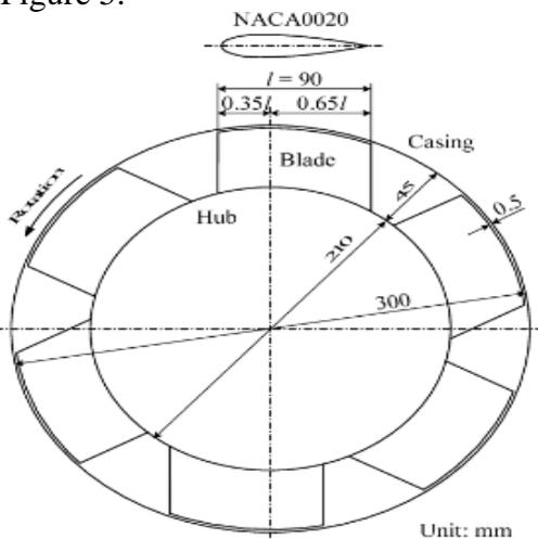
**Figure 5:** Tested wells turbine ( $D_w = 300$  mm)
