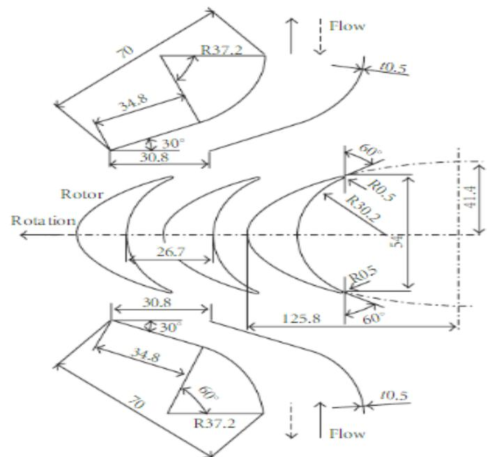
**Figure 6:** Tested impulse turbine ( $D_i = 300$  mm)
