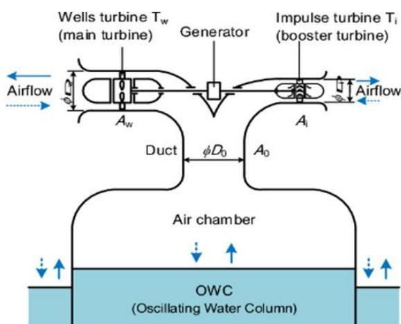
**Figure 3:** Principle of plant using wells turbine with booster turbine.
