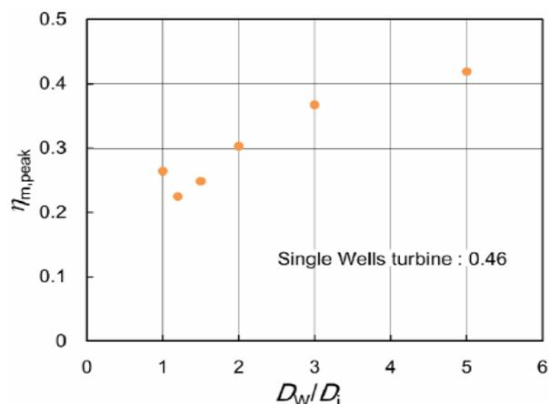
**Figure 10:** Effect of turbine diameter ratio on mean pinnacle efficiency.
