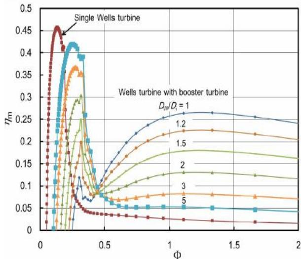
**Figure 9:** Effect of turbine diameter on mean efficiency under sinusoidal airflow conditions.
