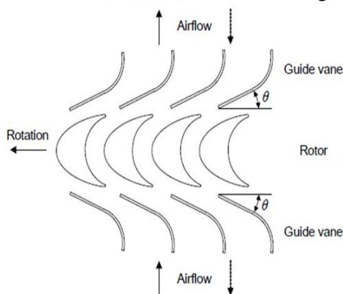
**Figure 2:** Outline of impulse turbine for wave energy conversion.
