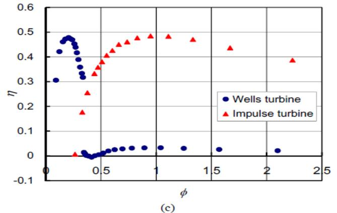
**Figure 7:** Turbine characteristic under unfluctuating stream condition: (c) Efficiency
