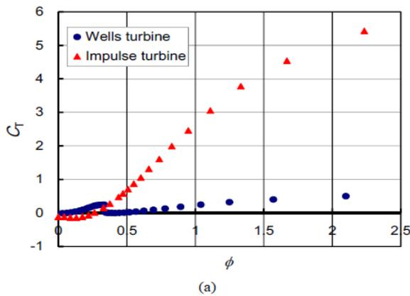
**Figure 7:** Turbine characteristic under unfluctuating stream condition: (a) Torque Coefficient
