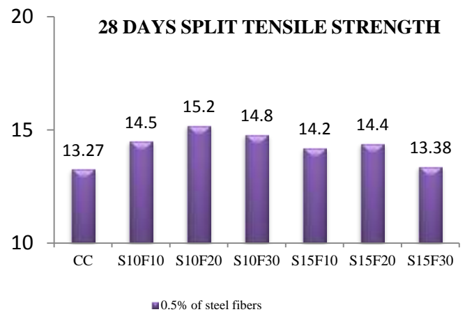
Fig: Tensile strength at 28 days for various percentages of Silica Fume and Fly Ash
