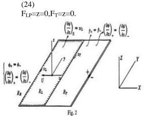
We shall designate the region occupied by the projection of the lifting surface by  $R_L$  and the region occupied by the trailing surface of discontinuity by  $R_T$  (Fig. 2). From (20) follows that when  $a_0=\infty$  the differential equation is, for steady as well as for nonsteady motion,
