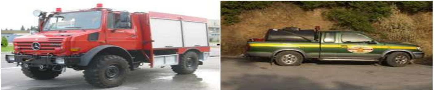
Fig. 6. Typical fire-fighting vehicle (Unimog of Elbo) and tank on 4×4 pickup.
