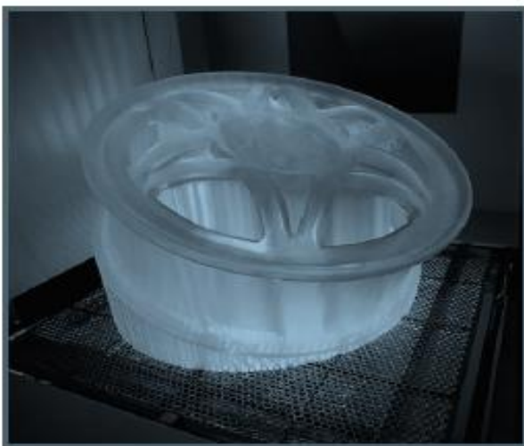
Figure 4: A part produced by stereolithography
