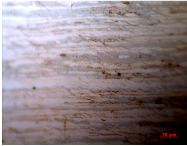
Figure 5: optical microscopy image of UNS S32205 duplex stainless steel sanded, polished, hydrogenated for 4h and degassed for 7 days, with a 500x magnification. Source: the author.
