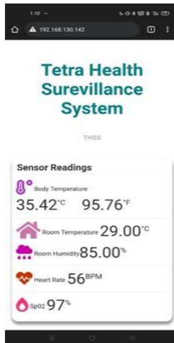
Figure 4 Output of Tetra Health Surveillance System (THSS)
