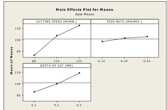
Fig.2—Effects of process parameters on radial force (raw data)
