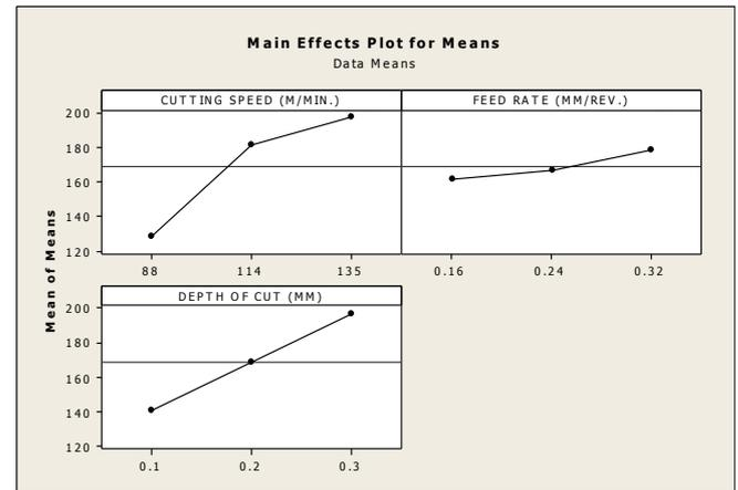
Fig.1—Effects of process parameters on axial force (raw data)
