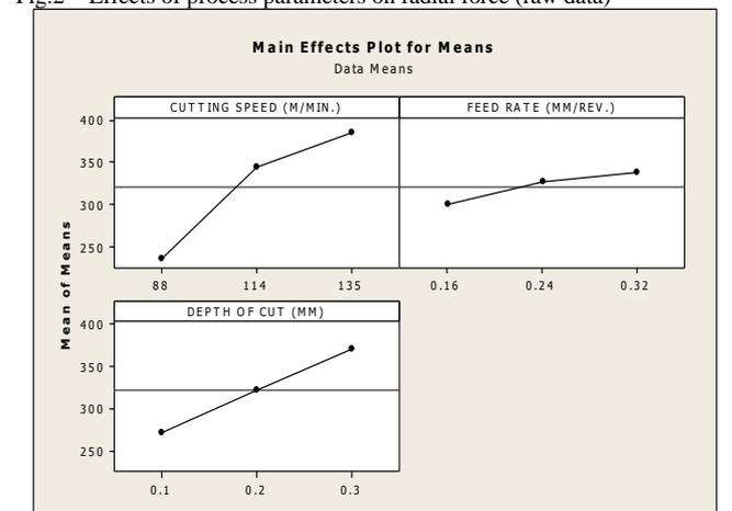
Fig. 3- Effects of process parameters on cutting force (raw data)
