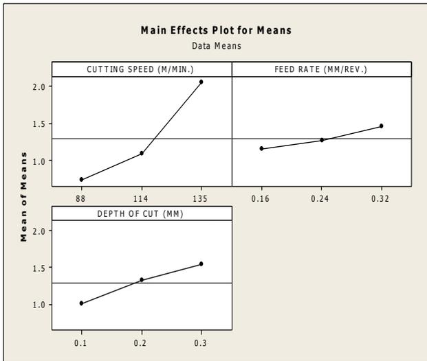
Figure 4: Effects of process parameters on MRR (raw data)
