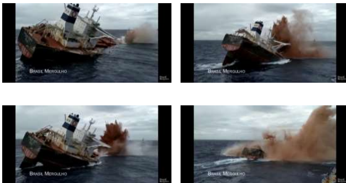
Scuttling of the vessel with successive flooding
