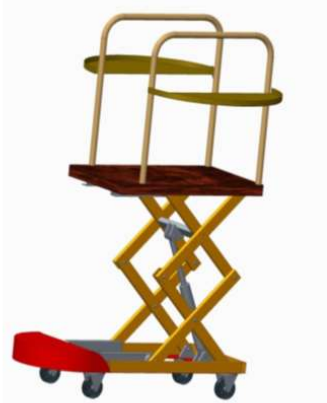
Figure 1(a): Platform at maximum extended position(3D design)
