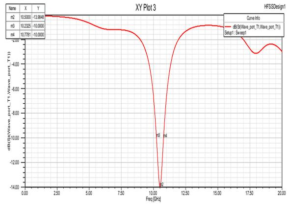
**Fig 2.** Frequency Vs return loss plot for rectangular patch antenna
