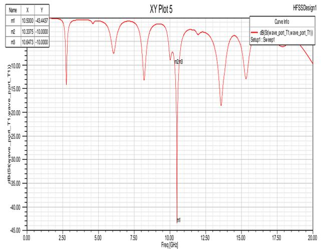
**Fig 6.**Frequency Vs return loss plot forCircular patch antenna
