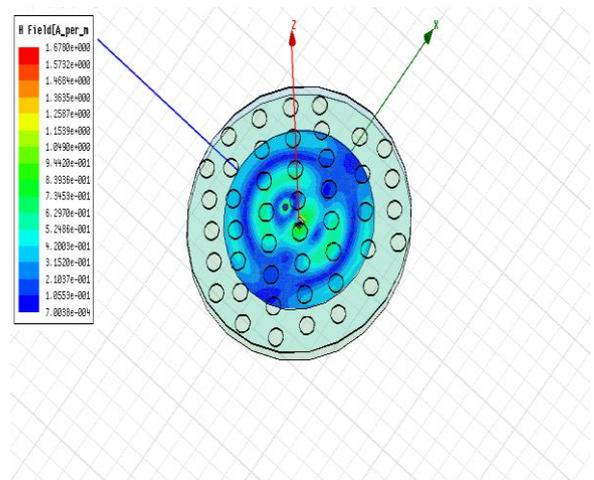
**Fig 8.**Magnetic Field distribution for circular patch antenna
