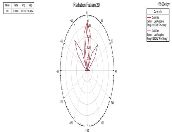
**Fig.7** Radiation Pattern for Circularpatch antenna
