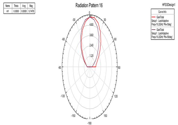
**Fig 3.** Radiation Pattern for rectangular patch antenna
