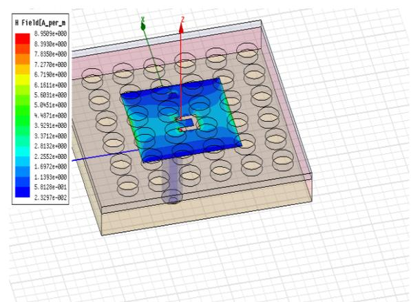
**Fig 4.** Magnetic Field distribution for rectangular patch antenna
