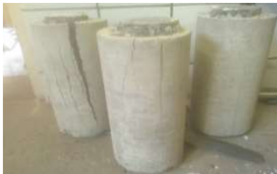
Figure 1: Failure of sections after testing
