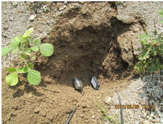
a. Buried sensors
