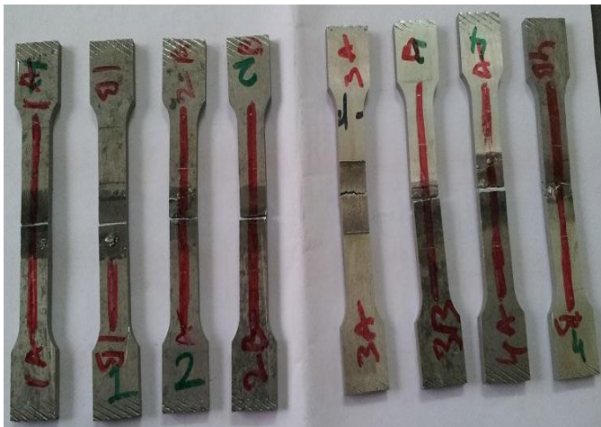
Fig9: Specimens after tensile testing
