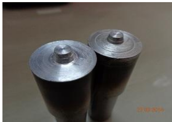
Fig5: FSW tools after welding
