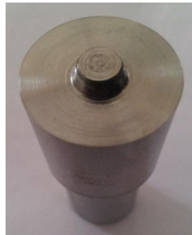
Fig4: FSW tools before welding
