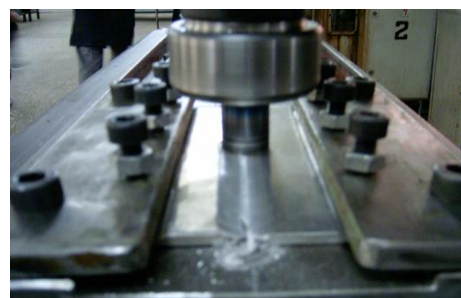
Figure1: Schematic illustration of welding of the different aluminum alloys
