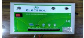
The batteries used in the fridge are rated at 12 volts DC, 7.5 Amphrs. To charge these batteries from the solar panel, a charge controller rated 12 volts, 10 amps is used as shown in the figure.
