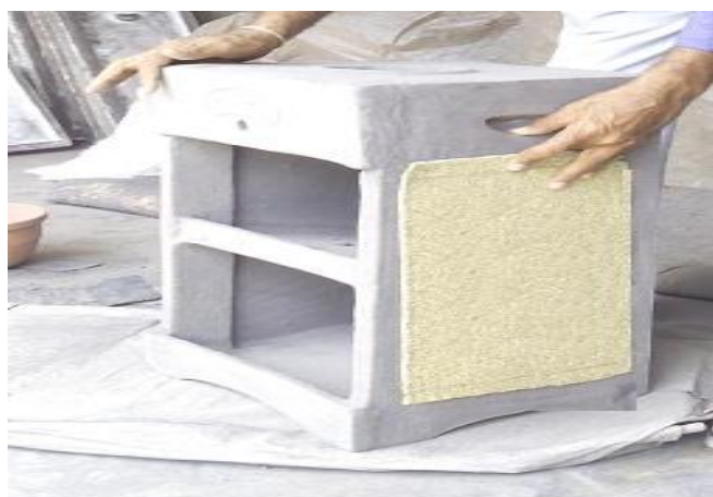
Figure 9: Luffa Cylindrica Insulation sheet attached to Mitticool Fridge
