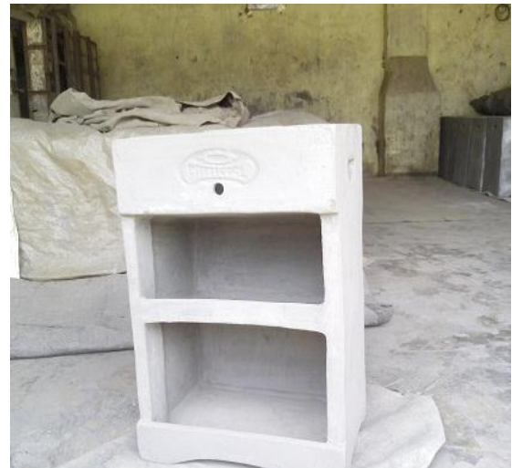
Figure 5: Raw Mitticool Fridge before sending to Oven
