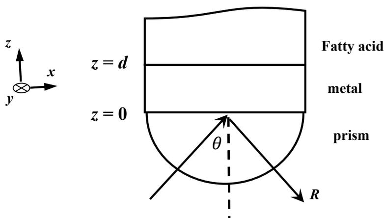
**Figure 1.** Geometry of the ATR The incoming waves propagated into a high index prism. Total internal reflection at the base of prism at  $z = 0$  generating evanescence waves. Then, this evanescence waves travelled to the interface between metal-fatty acid to excite surface phonon. This interaction decreased the ATR reflection  $R$ .
