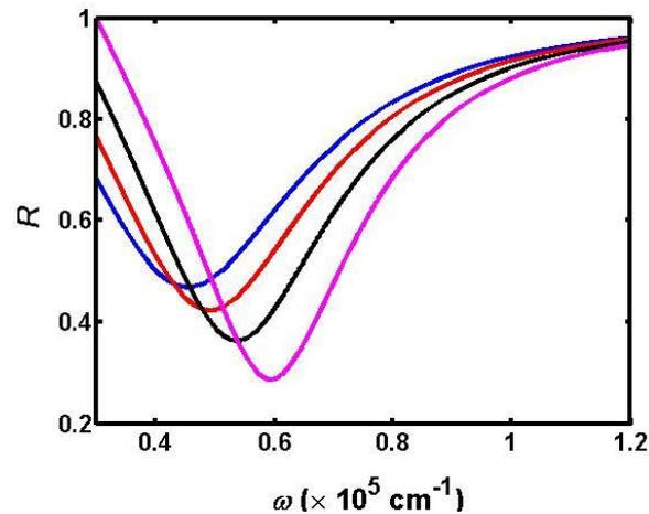
**Figure 2.** The calculated ATR spectroscopy of surface plasmon generated at the interface of gold-fatty acid. Here, we vary the value of fatty acid's permittivity. Magenta for  $\epsilon_f = 2.2$ ; black for  $\epsilon_f = 2.4$ ; red for  $\epsilon_f = 2.6$  and blue for  $\epsilon_f = 2.8$ . It can be noticed that each curve had similar trend, with the dips around  $\omega = 0.5 \times 10^5 \text{ cm}^{-1}$ .
