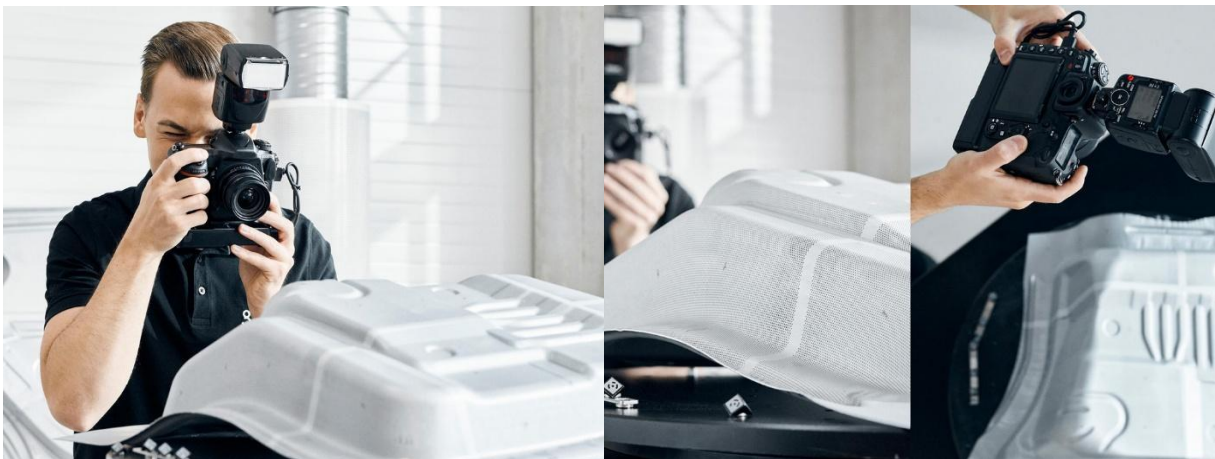
Fig. 1. ARGUS optical forming analysis in use: A technician photographs a stamped panel with the calibrated ARGUS camera. The part's surface was prepared with a fine etched dot grid, enabling precise measurement of deformation after forming. The system uses photogrammetry to determine 3D coordinates of the part surface from multiple images. Each dot's movement from its original grid position yields the local strains.[8]
