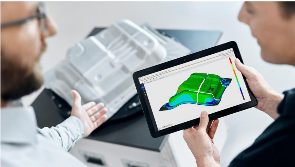
Fig. 2. Example ARGUS output for a formed part: (a) Full-field major strain distribution on an automotive panel, measured by ARGUS. Warmer colors (yellow/red) indicate higher strain areas; cooler colors (green/blue) indicate lower strain. (b) Forming Limit Diagram (FLD) for the same part. Each point represents the major/minor strain at a location on the part. The red line is the Forming Limit Curve for the material. Points below the line (mostly green/blue points) are within safe deformation range, while any points above would indicate localized over-strain (risk of necking/split). In this case, all measured points are beneath the FLC, signifying a successful forming without splits.[8]
