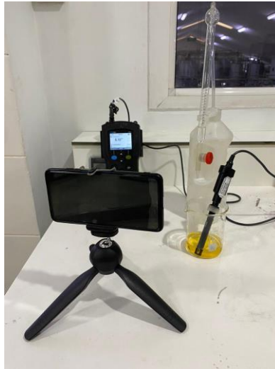
Fig. 1 : Alkalinity determination : pH-titration assisted by Smartphone video
