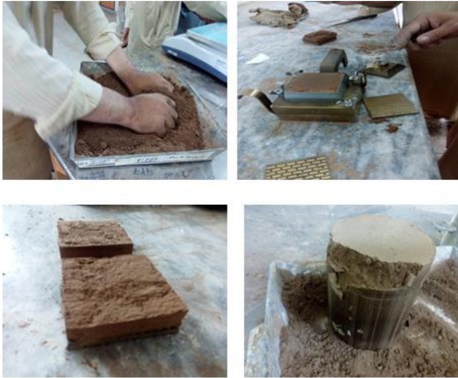
Figure 54: shear box sample
