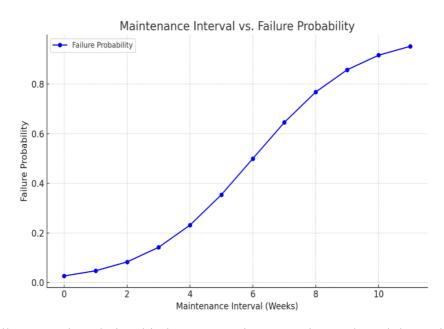
The graph above illustrates the relationship between maintenance intervals and the probability of equipment failure. As maintenance intervals increase, the failure probability rises, especially beyond the optimal interval of around six weeks in this example. This insight can help companies find the right balance between maintenance frequency and risk, thereby optimizing schedules for both cost savings and operational reliability.
