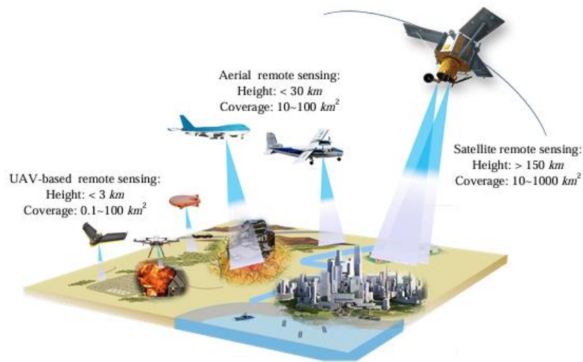
Figure.3. Remote sensing platforms of satellite, manned aviation and low-altitude UAV (Xiang et al.,2018).
