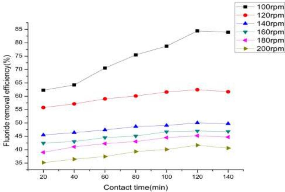
**Figure.3.** Effect of rpm on fluoride removal efficiency
