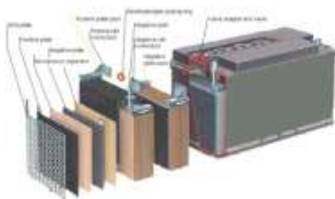
Fig3.4 Constructional block of lead acid battery
