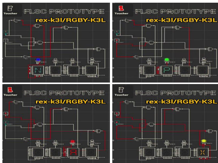
Figure 7: Experimental verification of the four logic states: N (Blue), P (Red), A (Green), and X (Yellow). Each panel confirms that for any input combination ( b_1, b_0 ), only one spectral output is active, ensuring a noise-immune representation.
