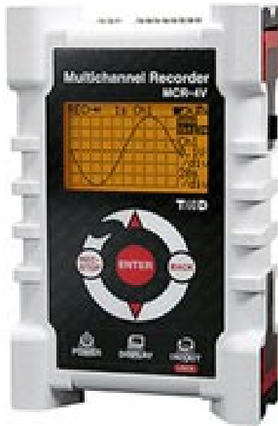
Figure 2.2 4-Channel Voltage Data Logger T&D Cooperation, 2015)
