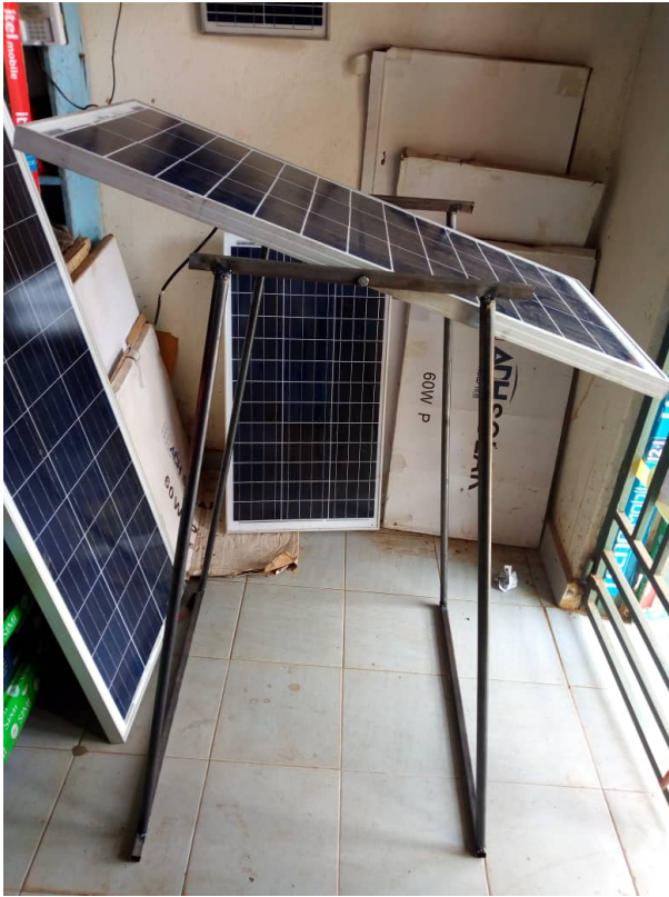
Figure 3.5 Constructed mechanical solar tracker
